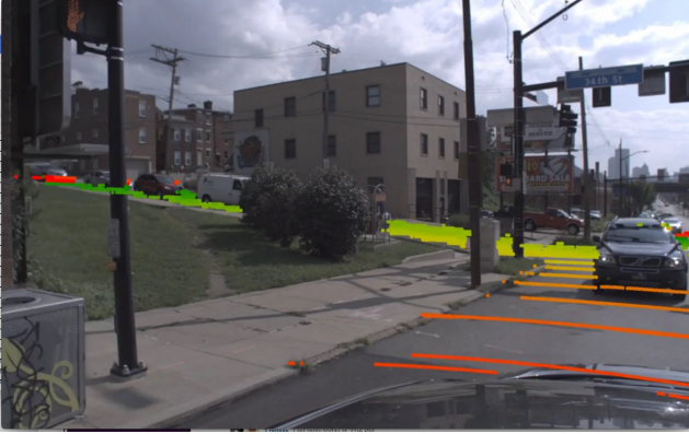
Figure 13: A scene with non-planar ground surface. The colored LiDAR returns have been classified as ground based on the map. Points outside the drivable area are also discarded. This simple distance threshold against a map works well, even on the road to the left which goes steeply uphill.
