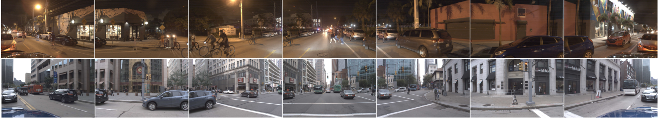
Figure 11: Ring Camera Examples. Scenes captured in Miami, Florida, USA (top) and Pittsburgh, Pennsylvania, USA (bottom) with our ring camera. Each row consists of 7 camera views with overlapping fields of view. Camera order is rear_left, side_left, front_left, front_center, front_right, side_right, rear_right
